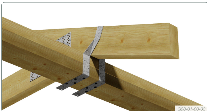
Cyclone Tie shown with each leg wrapped under the top plate and secured using 4/30mm x 2.8Ø Multinail nails.
