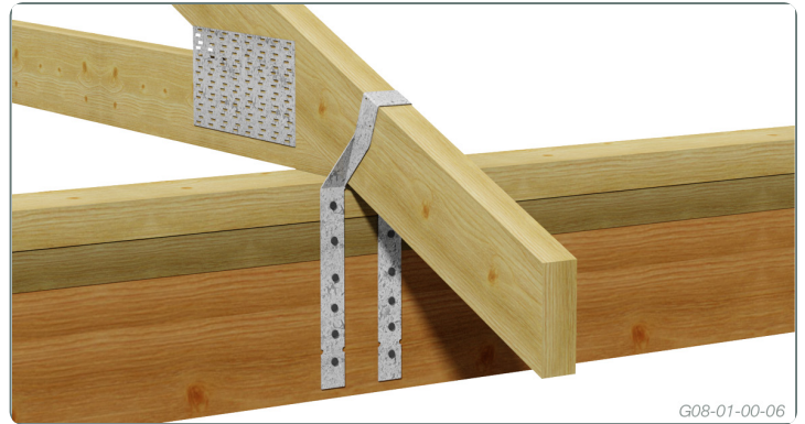
Cyclone Tie shown with each leg nailed down the face of top plates and lintel, and secured using 6/gun-nails
