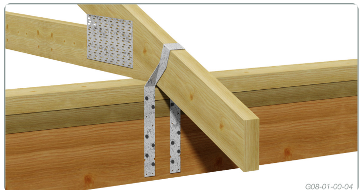
Cyclone Tie shown with each leg nailed down the face of the top plates and secured using 6/30mm x 2.8Ø Multinail nails.
