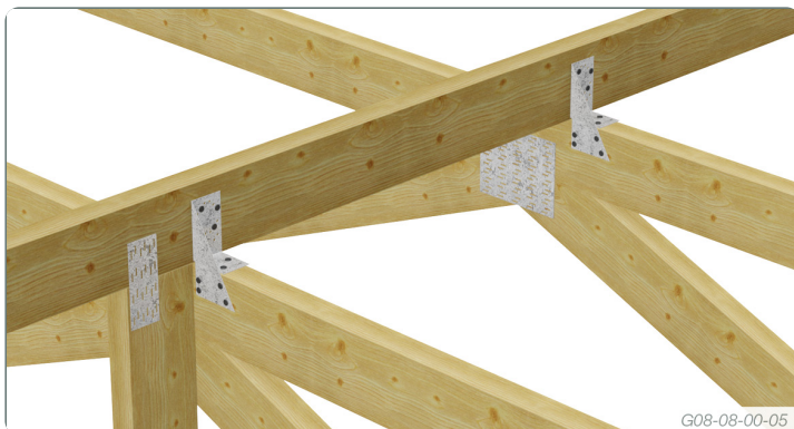
Jack flyovers to truncated truss
