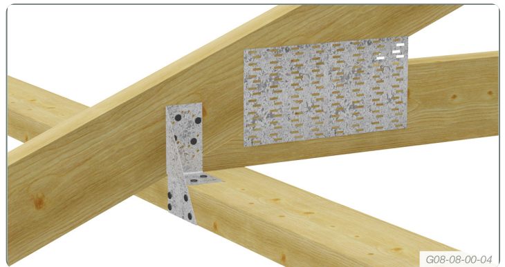
Connecting of Roof Trusses to Wall Plate.
