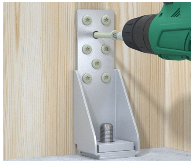
Figure 3 Fix the bracket to the vertical timber element using Multinail Advance 8mm Pan head screws with adequate torque
