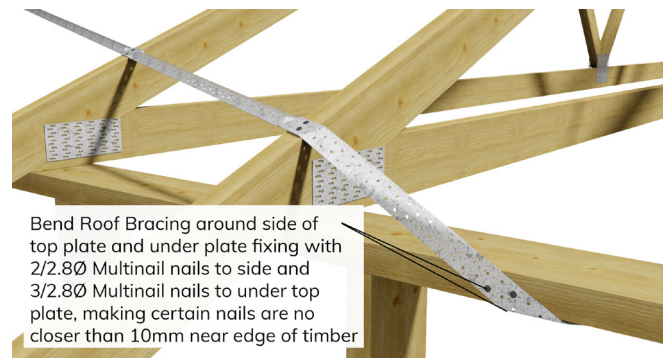
Figure 2: Heel End Fixing Detail
