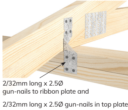
Figure 2: Uni Tie tie-down roof truss to wall frame at 90 degrees
