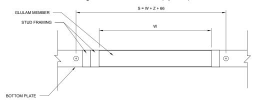
W = SIZE OF GLT MEMBER INCLUDING TOLERANCE (200-600mm)
