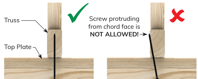
Figure 10: Correct vs incorrect installation
